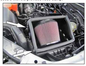
11. Install the filter/heat shield assembly onto the lower air filter housing and secure with the factory retaining clips.
