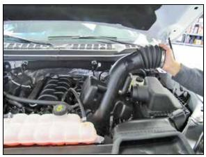
4. Unhook the coolant line from the intake tube and then remove the intake tube from the vehicle. NOTE: K&N Engineering, Inc., recommends that customers do not discard factory air intake.
