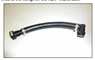
15A. On some later models it may be necessary to assemble the crank case vent hose assembly with the provided parts and install due to the manufacturer changing the position on the valve cover port. Install the assembly with the 90° fitting attached to the valve cover port.
